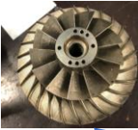
Compressor impeller PM Rotor, Tie bolt
